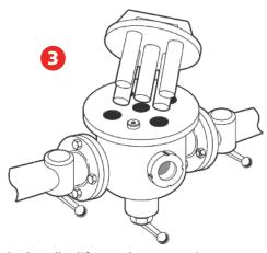
Using the handle, lift out the magnetic cores to remove from stainless steel housing. Take care not to knock or drop the magnetic cores as this can result in damage.
