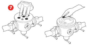
Replace the magnetic core and tighten the black retaining knob - Hand tighten only.
