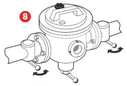
Re-open full bore isolation valves to complete the process. Use the *MagnaClean Industrial* isolation valve to remove the air from the unit.
