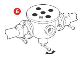
Close the drain point, i.e. turn off the drain valve or replace the plug.
