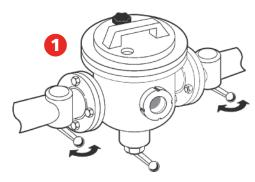
Check the MagnaClean Industrial sight glass for build-up of black iron oxides. If needed, turn off the boiler and isolate the electrics. Turn off the full bore isolation valves on either side.
