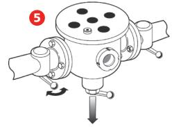
Slightly open the inlet isolation valve, leaving the other valve closed, and allow the deposits to drain through.
